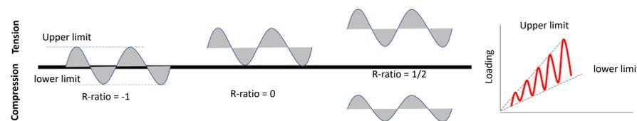
The concept of additive fatigue damage states that the same percentage of cycling to failure generates the same amount of internal damage, regardless of the applied loading. The fatigue life can be compared to a battery containing a certain amount of charge. Life can be consumed quickly at high load and slowly at low load. Consuming a third of its charge could happen quickly or slowly but provides the same end result: a remaining two thirds.
