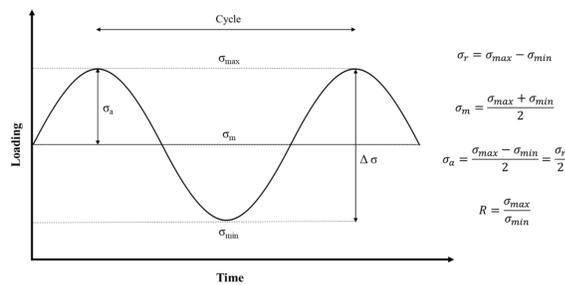
Lab convention for fatigue testing is to use a constant r-ratio (typically 0.1) when generating an entire S-N curve to simplify documentation and S-N curve comparison. A constant r-ratio removes the need to document the minimum load/stress for every specimen tested.
