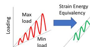
$$\text{Strain Energy} = \frac{1}{2} \times \frac{1}{E} \times \sigma^2 \quad \longrightarrow \quad \frac{1}{2} \times \frac{1}{E} \times \sigma_1^2 = \frac{1}{2} \times \frac{1}{E} \times \sigma_2^2$$
