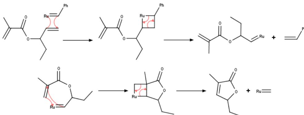
Figure 3. Ring closing metathesis of Grubbs' catalyst.
