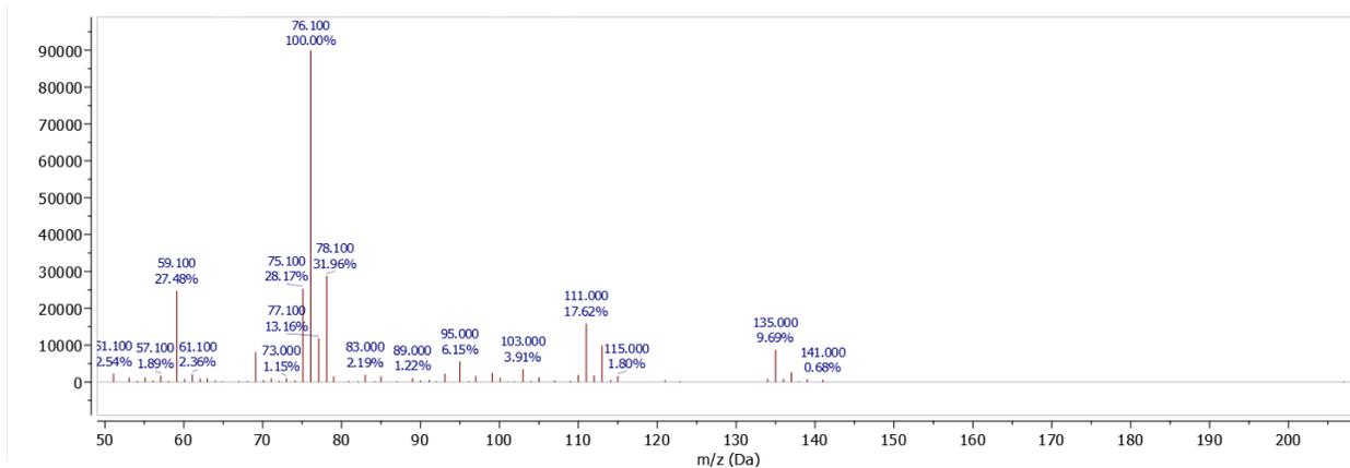
Figure 5. Mass spectrum of Methacryloyl chloride at 5.905 min.
