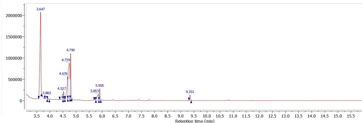
Figure 4. Total Ion Chromatogram (TIC) of Methacryloyl chloride.
