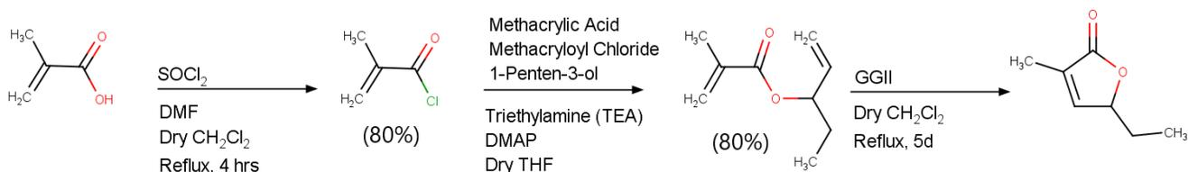
Figure 2. Reaction scheme of synthesizing an acyl chloride, ester, and butenolide.
