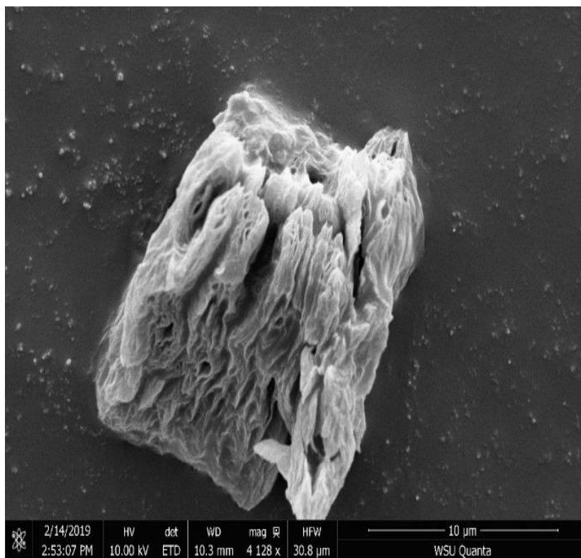
Figure 3. SEM images of Co/GO dispersed on a carbon stub and after sputtering with Au. This image was captured utilizing a FEI Quanta 250 SEM. The layered sponge-like porous morphology of the material provides a higher surface area lowering the amount of metal loading. This image was taken at a distance of 10 μM.
