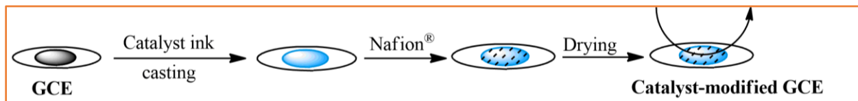
Figure 2. Experimental setup of electrode modification plan.
